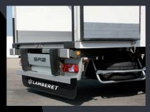
Reinforced rear protection system: Large vertical buffers at the end of the side threshold and elastomer-stainless steel shock absorbing buffers on the chassis.
