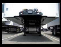
Front module with integral decking without recessing, ensuring the robustness of the body-chassis connection at the level of the coupling and optimising the available usable height: 2.70 m with R65 tyres, whilst remaining within the 4 m overall.
