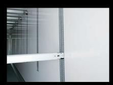
Duplex Pack: System with recessed vertical rails in the lateral surfaces and bars able to support 1000 kg allowing palettisation on 2 levels (66 euro pallets).
