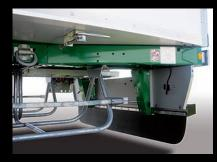
Treatment of the chassis by shot blasting and powder coating, 6 year anti-perforation warranty. Possibility to match the colour of the chassis with your colour scheme (100% of the RAL colour chart available).
