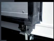
High performance single-piece seal Single-piece frame seal on the door profile in pultruded composite (resin and fibreglass), impervious to variations in temperature. Its 8 lips are equipped with ridges improving water tightness.
